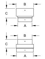
Designed to increase or reduce the size of an EXCELiner to accommodate a range of flue sizes, appliances and installations. Note: Increasing or decreasing chimney size can have a negative impact of chimney performance and safety. Use these components only when appropriate.
