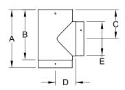
EXCELiner tees are made from .025" thick stainless steel. The removable snout is fastened to the body of the tee with heavy duty stainless steel screws. All 5 1/2", and 6" tees have a 6" diameter snout so that they can connect to 6" smoke pipe without a reducer. Tee Cap (LTC) not included.
