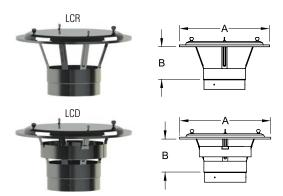
EXCELiner rain caps are made entirely of type 304 stainless steel. The top is held in place with four wing nuts on the regular (LCR) and deluxe (LCD) rain caps for easy removal and cleaning without the need to remove the rain cap itself. The deluxe cap has a stainless steel band.
