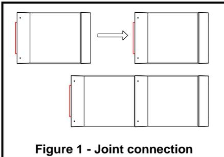
The outer casing of EXCELDirect® is tapered to make connection easy. Simply slide one length onto another and press firmly. The inner liner joint will be automatically sealed. Once the lengths are firmly joined, fasten the joint with the three #6 x 3/8" screws provided. All lengths are assembled this way.
