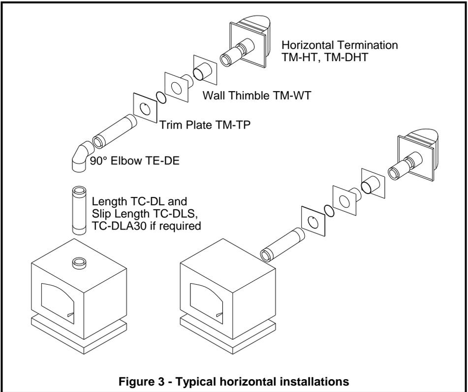
**Figure 3 - Typical horizontal installations**
