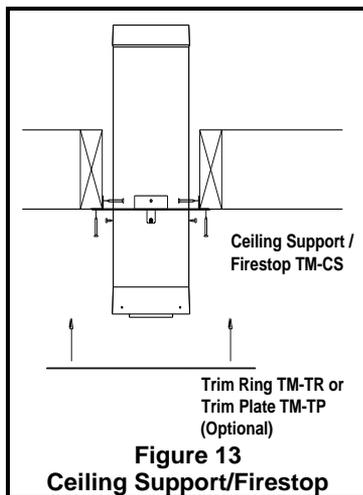
Pass the venting through the support and then fix the support to the pipe with the three tabs that were previously bent downwards. Use the screws provided.
