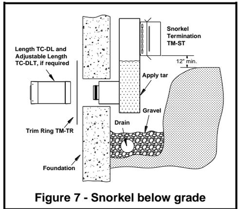
If the base of the snorkel is below grade (i.e. basement installation), proper drainage is required to prevent water from entering in the snorkel. The portion of the snorkel that is below grade must be coated with tar to prevent corrosion. See Figure 7.
