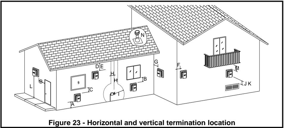
**Figure 23 - Horizontal and vertical termination location**
